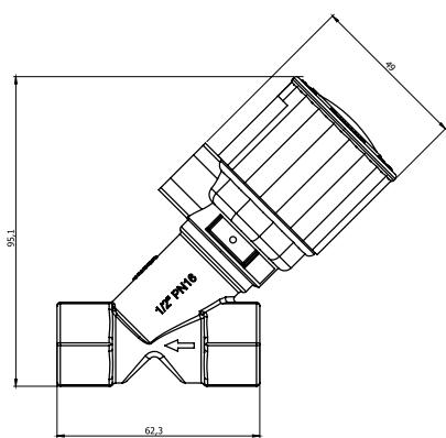
Opposite flow direction prevents the leakage of the fluid by the pressure in the inlet pushes the plunger. The problem of leakage with the increase of the inlet pressure is a problem that is constantly encountered in other piston valves. However, this time, if the flow
