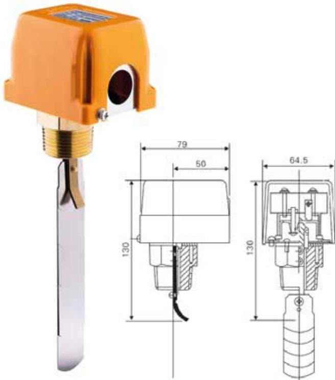
It is suitable for water, cooling systems, lubrication systems, and fire systems. PFS Series flow switches, equipped with various sizes of paddles, can be used for flow/no-flow detection and providing contact for low or high flow applications in pipes ranging from 1" to 6" in diameter.
