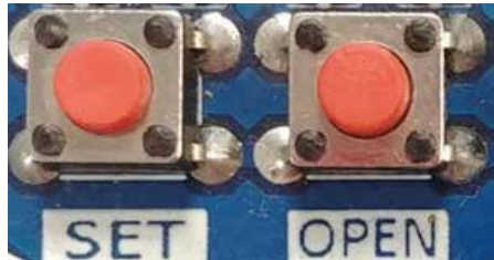
Figure 15. Buttons used for automatic calibration
