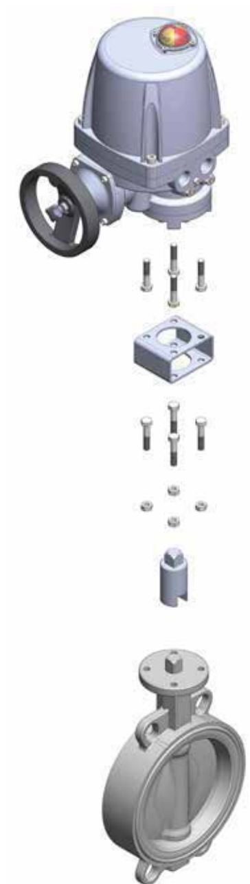
Figure 6. Mounting the Electric Actuator to the Valve with Bracket
