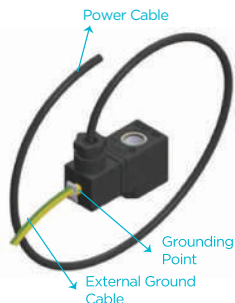
Figure 8. Ground connection of ex proof solenoid coils
