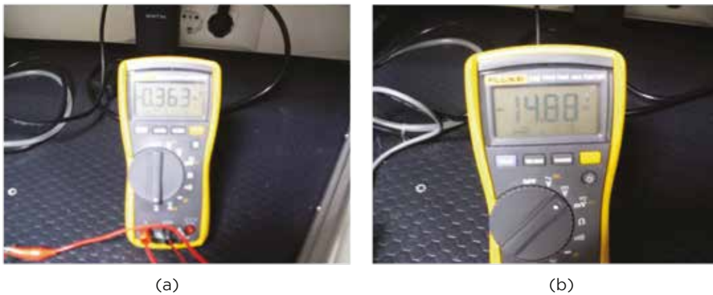
Figure 7. Measured Values on the Coil: (a) Current Value, (b) Voltage Value.
